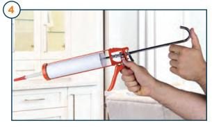
Move push rod hard against cartridge plunger. Cut cartridge and nozzle as required and depress trigger to commence gunning.
