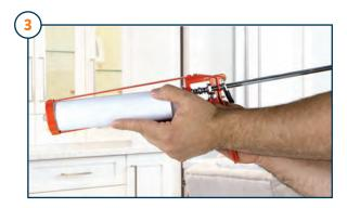
Insert cartirdges as indicated. Ensure front of cartridge is placed securely within the guns end ring.
